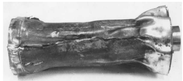
Fig. 2. The shell, obtained when using the first technological scheme welding
